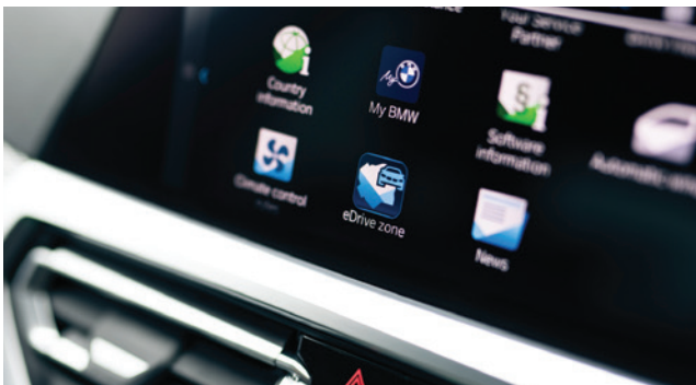
The BMW eDrive Zone technology automates the process of switching to electric-only power when a BMW plug-in hybrid vehicle enters a defined area of a city.
